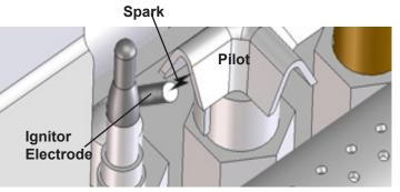
Pressing the ignitor button should produce a spark between the ignitor electrode and the pilot where shown above.
