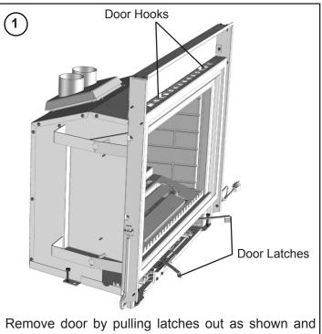
Remove door by pulling latches out as shown and pulling the bottom of the door out from the unit about 3". Then lift the door slightly up and off the hooks.
