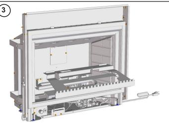
Remove air plate by lifting it up about 3 inches and then out of firebox. Be careful not to damage side brick panels.
