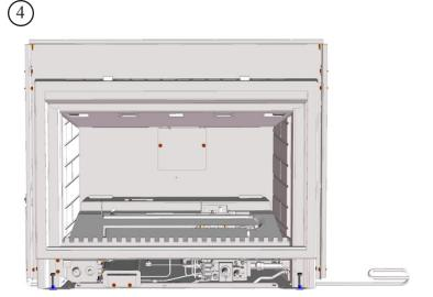
Remove 2 screws holding exhaust cover plate onto the rear of the firebox and remove cover.
