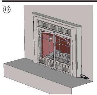
Install the face doors by hanging them on the hinges. **Note: a brass washer goes between the hinges.** The finished installation should look like this.
