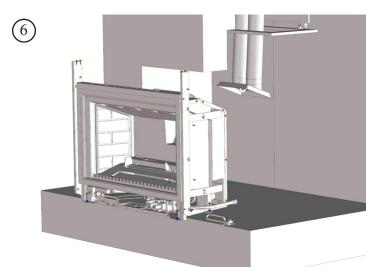
Determine the flue restrictor needed for this application and install into the exhaust pipe on the stove adapter.
