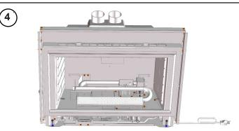
Remove the screws mounting the intake air deflector and lift it from the firebox. Next locate the screw holding the burner tube to the firebox floor and remove it. Now the burner orifice can be removed using a 1/2" deep well socket and replaced with orifice required for type of fuel being used. Refer to safety label for orifice size.
