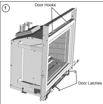
Remove door by pulling latches out as shown and pulling the bottom of the door out from the unit about 3". Then lift the door slightly up and off the hooks.
