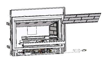
Remove the screw, washer and spacer from the center of the rear brick panel. Using one hand, gently push out on the side brick /relief door to allow clearance for removing the rear brick panel.
