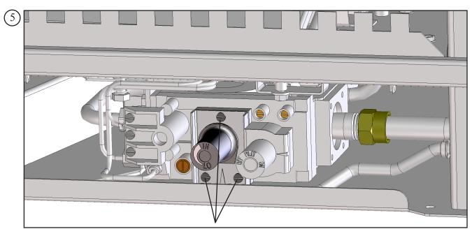
Remove three screws to change knob assembly. Install NG knob assembly in place of the LP assembly. Be sure screws are tight.
