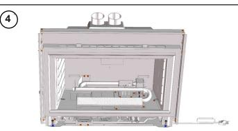
Remove the screws mounting the intake air deflector and lift it from the firebox. Next locate the screw holding the burner tube to the firebox floor and remove it. Now the #50 LPG burner orifice can be removed using a 1/2" deep well socket and replaced with a # 31 natural gas orifice.
