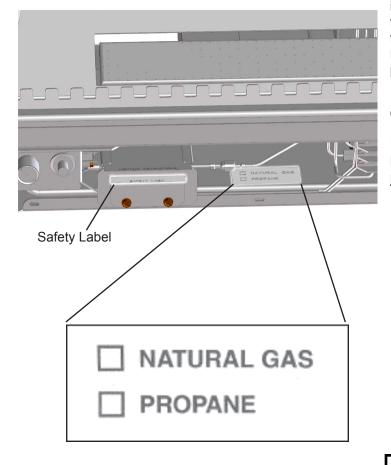
Place conversion sticker (provided in Kit) on the valve. This is to permanently mark the valve that it has been converted to Natural Gas. This label is important in the event that the valve is ever removed and mixed in with other valves. Reassemble all components removed during the conversion process.
