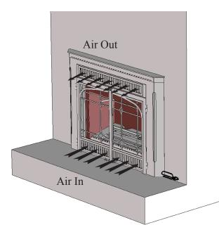
The flow of convection air must not be obstructed.
