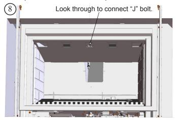
Check stove to opening side clearance. If there is not enough room to reach beside stove while it is installed you may want to remove the gas line from the valve assembly and connect it to your supply line inside the fireplace first, then reconnect to the gas valve.
