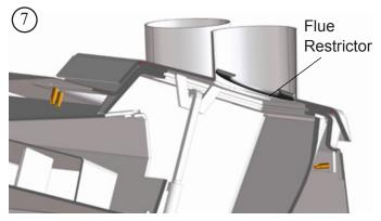
The flue restrictor can be installed after flex pipes are connected and stove is in fireplace opening. To change or install restrictor remove glass door then remove log. Next remove screw, washer and spacer in the rear brick panel and remove the brick panel while holding relief door open with one hand. Remove the 2 screws holding the exhaust cover onto the rear of the firebox.
