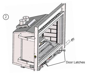
Open the glass door by pulling out on the 2 latches located on the bottom of the door frame. Pull the bottom out a couple of inches and lift the door off of the stove body and set safely out of the way. Remove the bag of rock wool, packaging materials and log set from inside the firebox.
