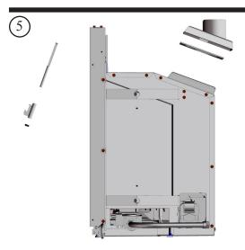
Using a 1/2" deep well socket loosen the nut that was under the exhaust cover plate until it is flush with the end of the threads. Pull the exhaust clamp down from notch in firebox top. Lift the clamp assembly up and disconnect it from the intake / exhaust adapter.
