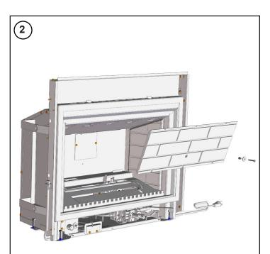
Remove log. Next, remove screw, washer and spacer from the center of the rear brick panel. Using one hand, gently push the side brick/relief door open slightly and using the other pull the top of the rear brick panel forward and remove it.
